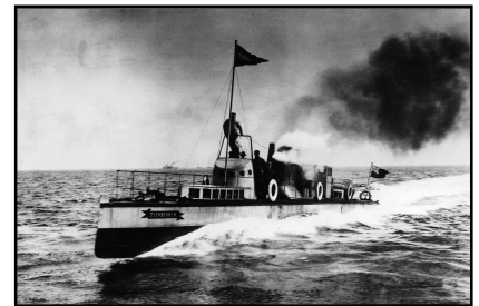
The classic photograph of Turbinia by Alfred West. Nearly 105 feet long, but just 9 feet across the beam, and a 3 foot draught (very similar dimensions to Goodheart), Charles Parsons' "ocean greyhound" Turbinia was the fastest ship in the world.
