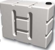
Constructed from a seamless rotationally moulded MDPE (Medium Density Polyethylene), which is semi-translucent, so the water level is easily visible through the tank. These tanks come complete with either ¾" (only 250 litre models) or 1" outlet at the bottom for connection to a tap or hose and an 8" vented cap. Other fittings can be supplied upon request (available separately).
