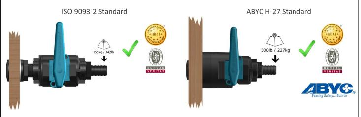
In accordance with **ISO 9093-2** standards, Skin Fittings (Thru Hulls) are subjected to a 155kg (341.7lb) load, applied to the threaded section for a minimum of 30 seconds, without any damage occurring. TruDesign Skin Fittings (Thru Hulls) meet this standard. Note:  $\frac{1}{2}$ " size Skin Fitting (Thru Hulls) are not approved to ISO 9093-2 or ABYC unless used with an ABYC collar.
