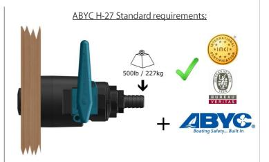
**TRUDESIGN**<sup>M</sup> Skin Fittings (Thru Hulls), when assembled together with **TRUDESIGN**<sup>M</sup> Ball Valves and Load Bearing Collars, comply with ABYC H-27 standards. This allows the entire assembly to withstand a 500lb (226.8kg) load applied to the inboard end of the assembly (i.e. from the Ball Valve's Tail fitting) for a minimum of 30 seconds without any damage occurring.
