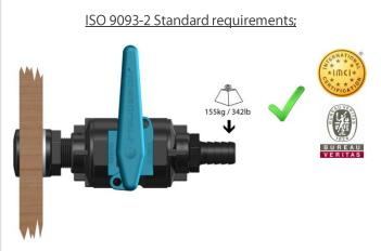
In accordance with ISO 9093-2 standards, Skin Fittings (Thru Hulls) are subjected to a 155kg (341.7lb) load, applied to the threaded section for a minimum of 30 seconds, without any damage occurring.
